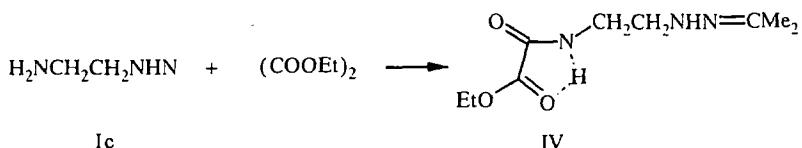
Formation of piperazine-2,3-dione does not occur either when heating compound IV or when treating it with base (sodium ethylate). Possibly the stability of the acylation product is due to stabilization (by the intramolecular hydrogen bond) of a conformation from which cyclization is impossible.
